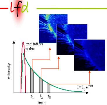
A sample is flashed many times by a short duration laser source
