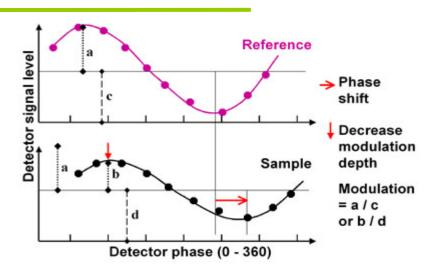
A sample is excited by a modulated light source
